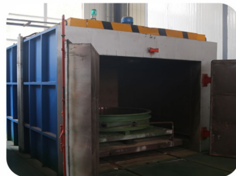
耐高温油漆固化炉 high temperature resistant paint curing furnace
